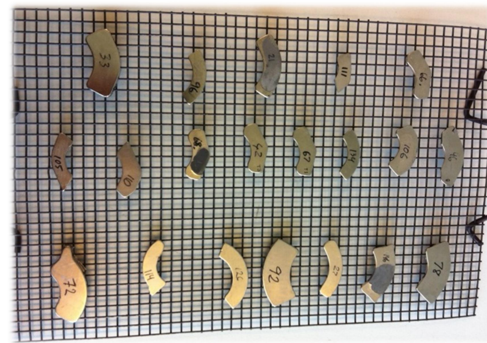
Figure 3: NdFeB magnets from HDDs analysed by EDX
